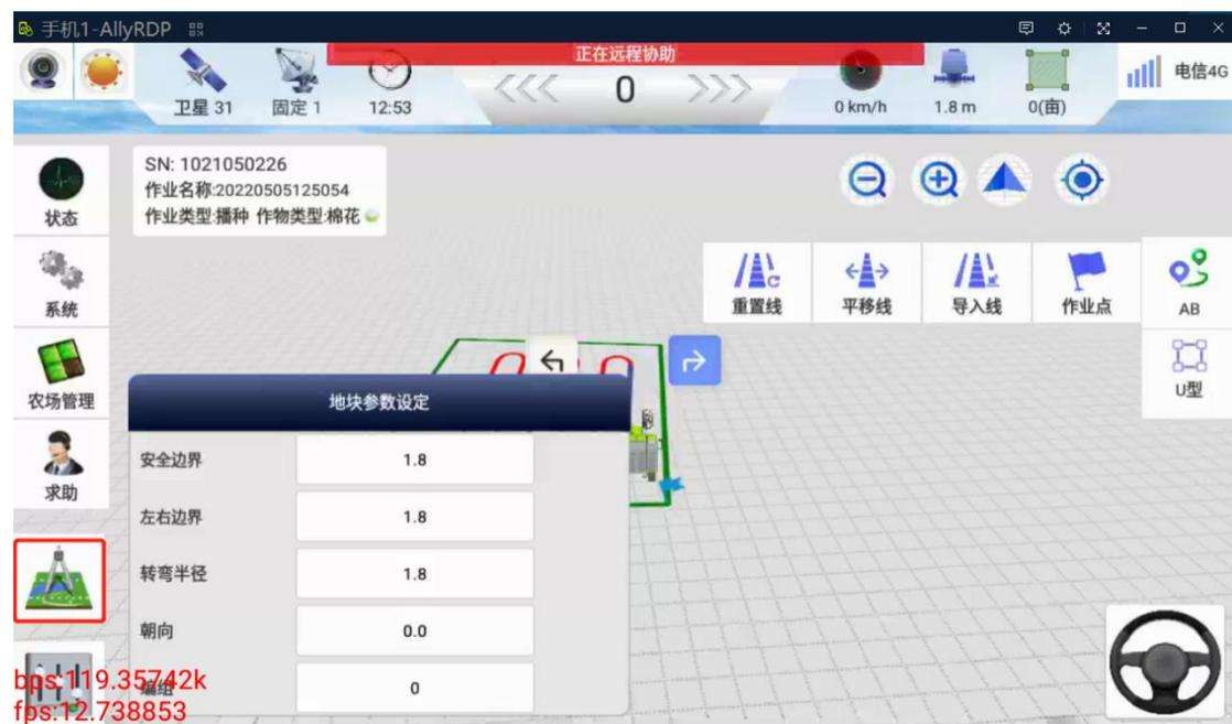
Then click the four-point planning pop-up window on the screen to set the safety boundary. The turning radius of ordinary high-speed riding rice transplanters is 1.8 meters, and the safety boundary is set to 1.8. The left and right boundary range can be set to 0.1~1.8, and the recommended setting value is about 0.5 meters to ensure safety.
