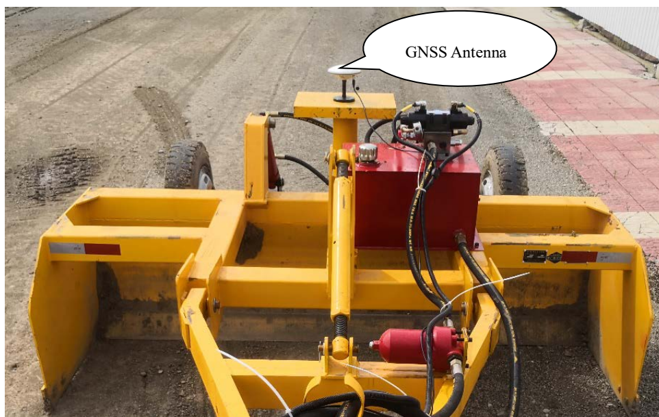
Figure 1 GNSS Antenna Installation
