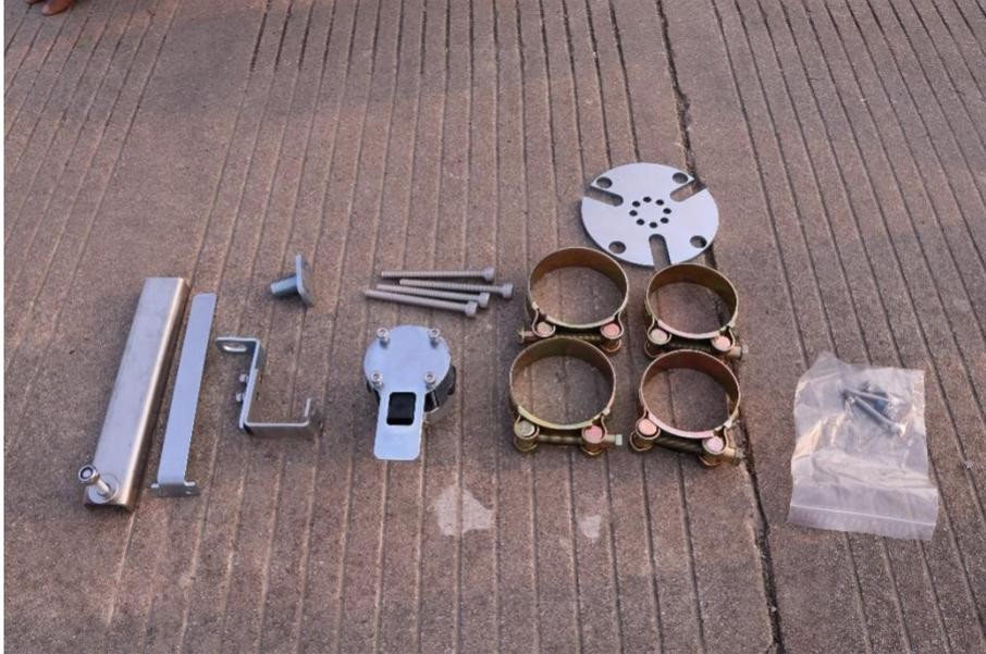
Figure 2.7 Components needed to install angle sensor
