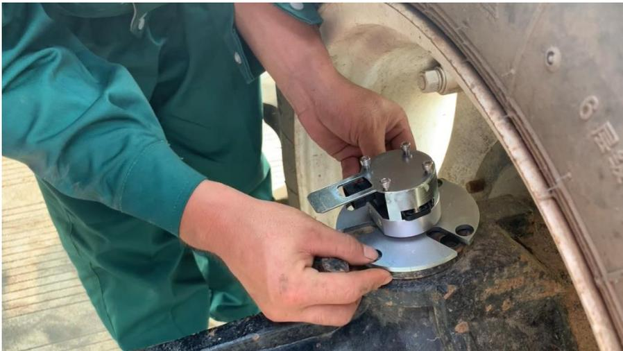
Figure 2.8 Install the parts to fixate angle sensor
