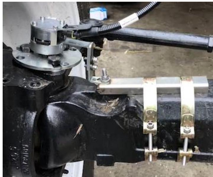
Figure 2.11 Installation example of angle sensor
