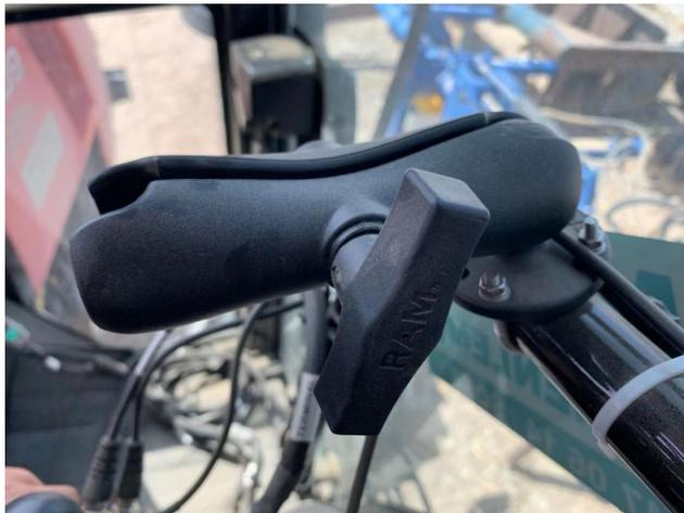
Figure 2.24 Bracket for T100 Control Tablet
