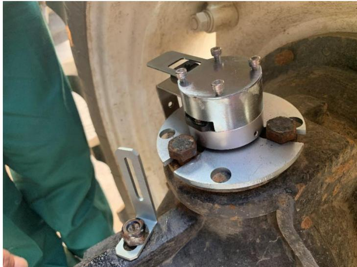
Figure 2.9 Possible position of angle sensor – 1
