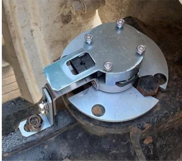
Figure 2.10 Fix angle sensor – 2
