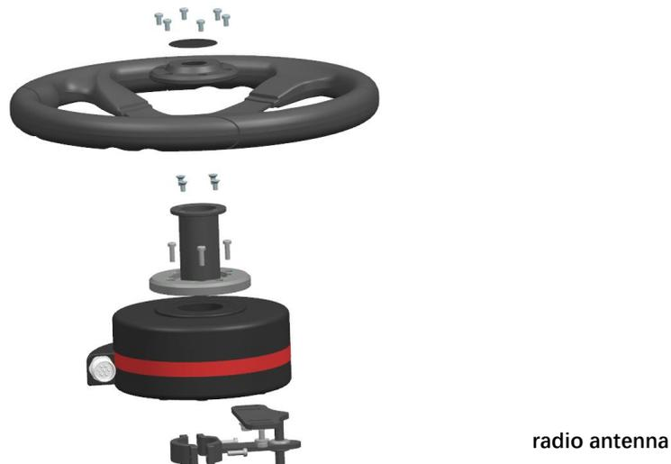
Figure 2.1 Assembly diagram of EMS2 motor wheel
