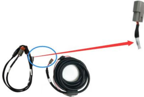
Figure 2 Power supply cable - main harness
