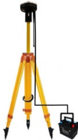
Figure 5 Mobile Base Station Installation
