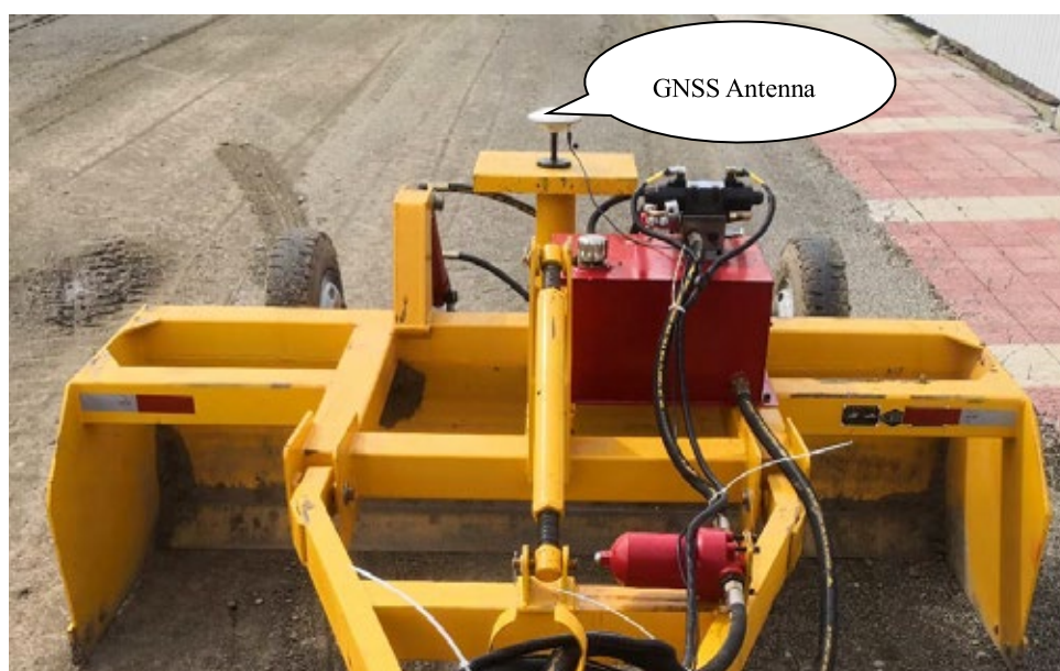
Figure 1 GNSS Antenna Installation
