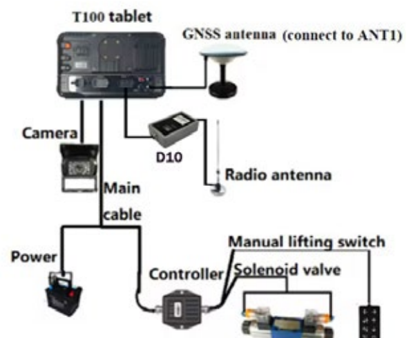
Figure 3 Cables Connection (with D10)
