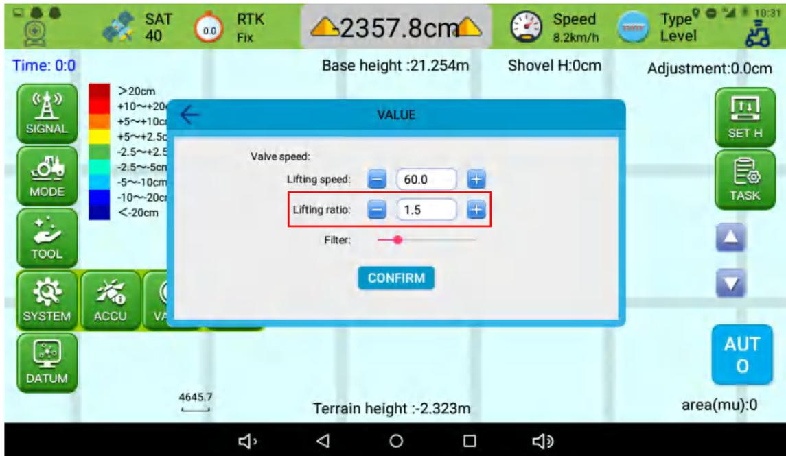
Figure 35 Adjust Lifting Ratio
