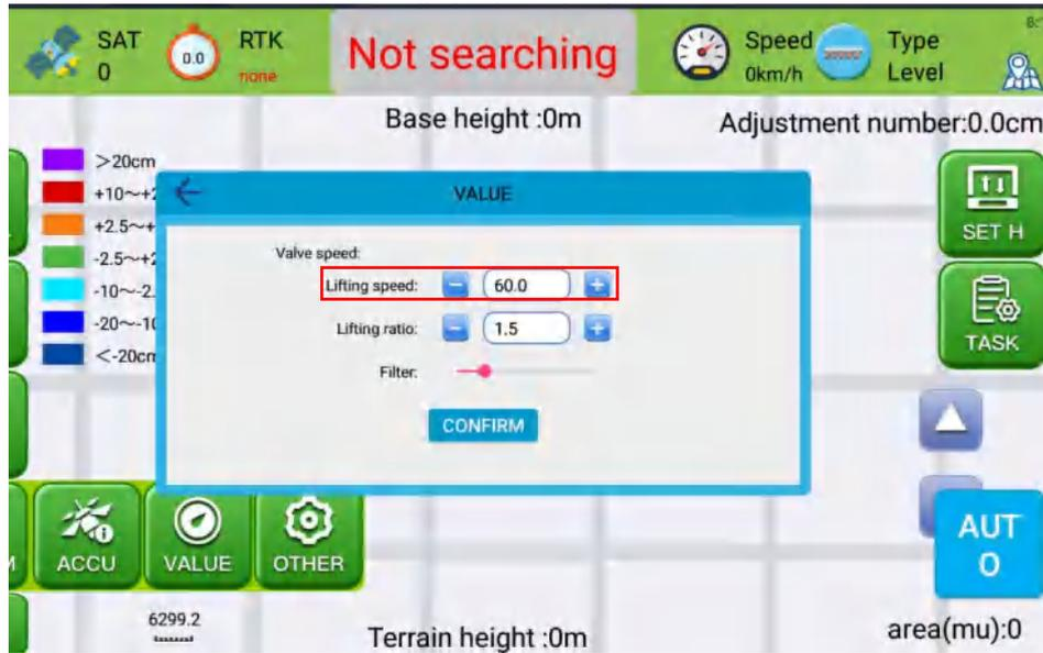
Figure 38 Adjust Sensitivity Value
