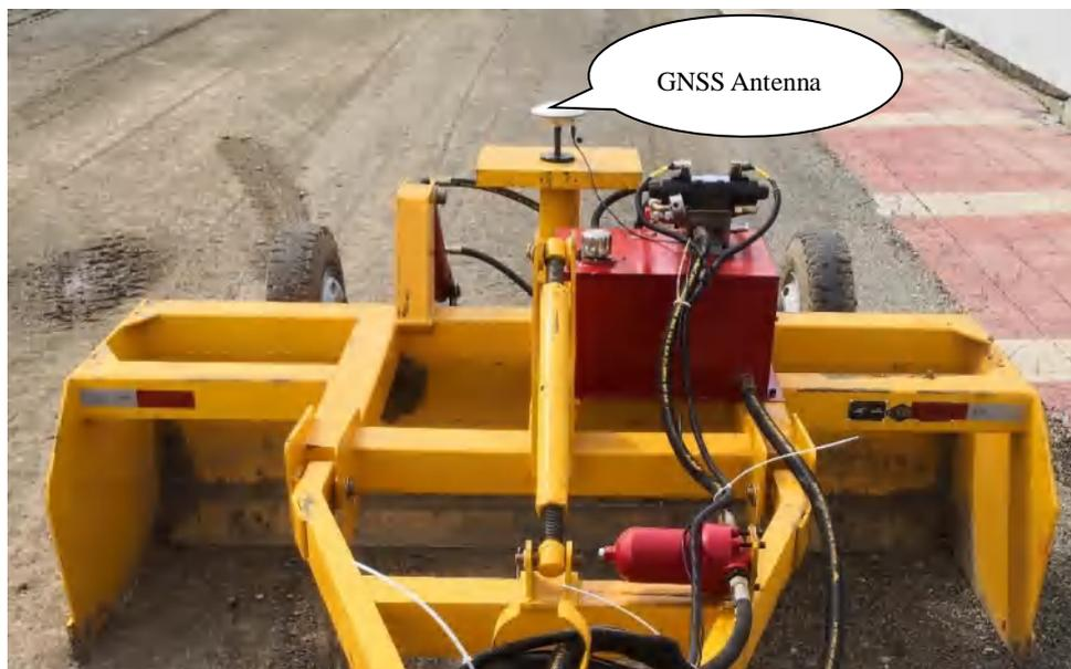
Figure 1 GNSS Antenna Installation
