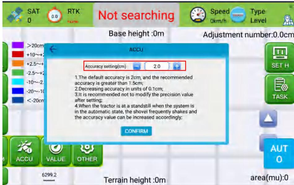
Figure 36 Adjust Accuracy Setting
