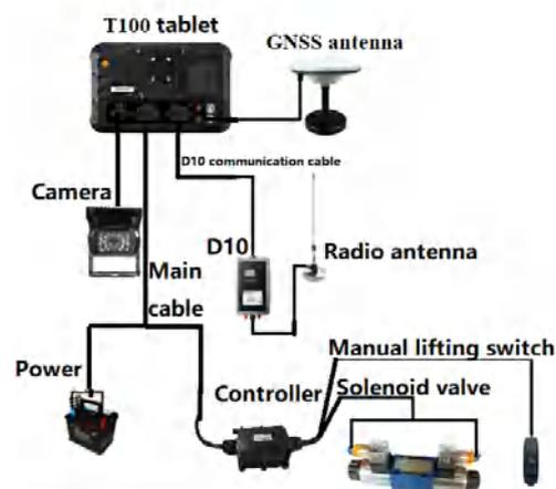
Figure 3 Cables Connection
